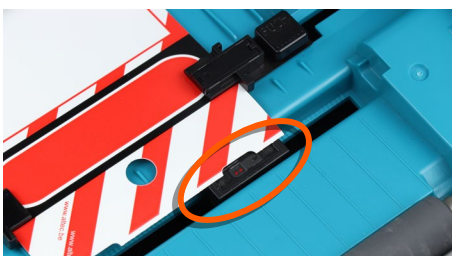
Labels with a notch out of range of gap sensor
