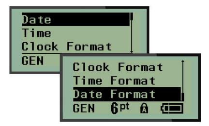
Figure 3 • Time/Date settings in Set Clock function
