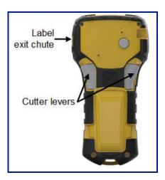
The label exit chute contains plastic grips that hold the label in place after cutting so it will not fall off.
