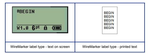
Figure 6 • Repeated data on a WireMarker label
