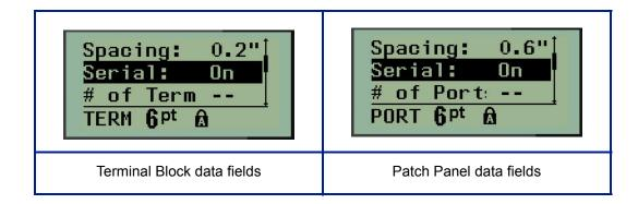
1. In the *Spacing*: field, enter the amount of space that exists between the terminals or ports.
